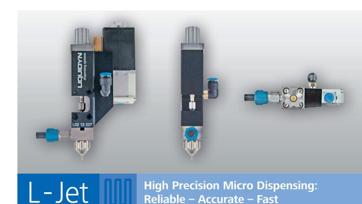
**High Performance Jet Valve:** For contactless dispensing low to medium viscous dispensing materials. Dispensing frequencies of up to 150 Hz allow for a faster production process. The fluid-carrying components are quick and easy to exchange – The separation of the actuator from the fluid-carrying components ensures a reliable dispensing process.
