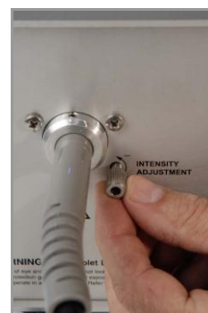
Intensity adjustment knob for fingertip adjustment
