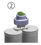
Whilst turning, the bajonett ring pulls the plug out of the cartridge.
