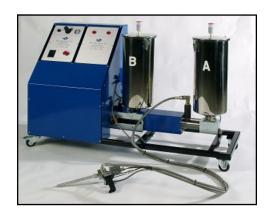
Metering Pumps: Single acting positive displacement.
