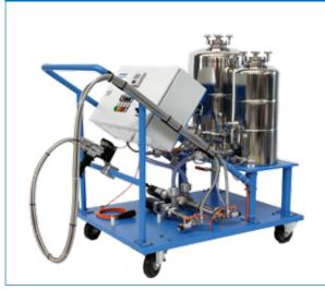
This compact, mobile version is highly suitable for the casting of low to high-viscosity materials. Both components are poured into separate tanks. The tanks are designed for pressurized as well as vacuum operations. Material is statically fed to two dosing pumps and then dosed through separate hose lines (approx. 3 m length) into the 2-component mixing head.
