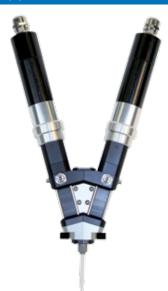
The 2-component dosing system ViscoDuo-V 4/4-EC is a valveless, static mixing head with dispensers located directly in front of the mixer. Especially developed for simplified cleaning (Easy Clean) and maintenance. In the mixing head no valves are required. The components to be mixed are dosed by volume only and with no dead space into the static mixer.
